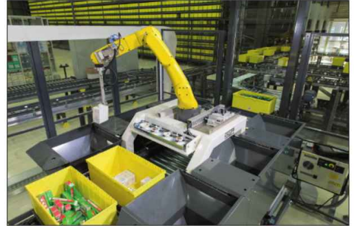
Pick-it-Easy Robot picks articles from the source container and transfers them to the target container.
