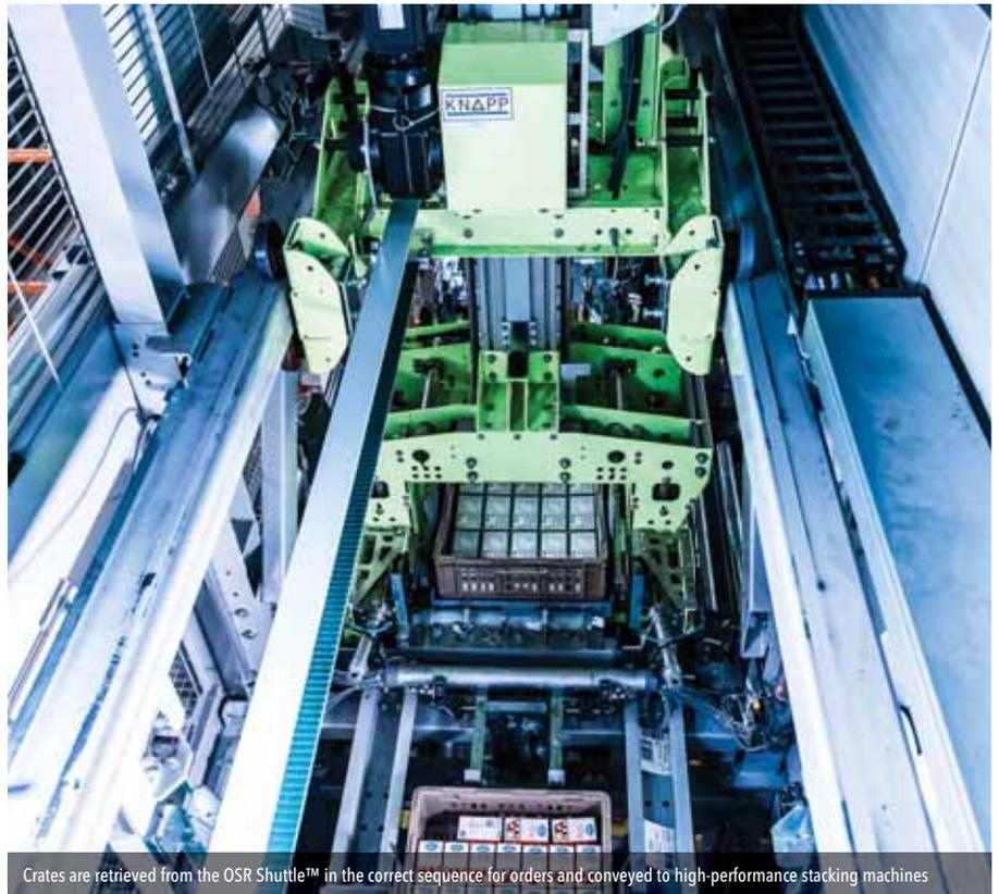
Crates are retrieved from the OSR Shuttle™ in the correct sequence for orders and conveyed to high-performance stacking machines
