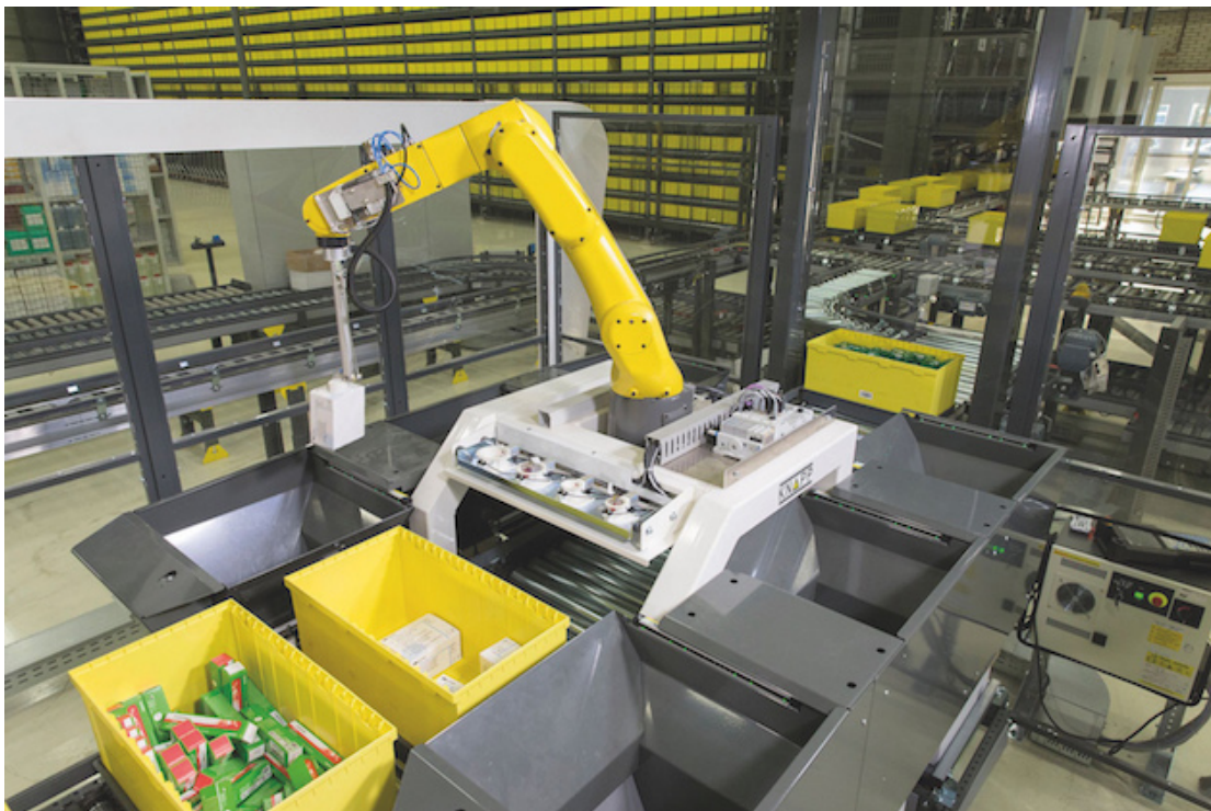
Pick-it-Easy Robot picks articles from the source container and transfers them to the target container
