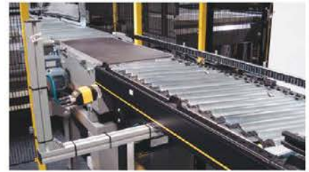
For the transportation of biscuit boxes from the different production lines to the palletizers, TBWB implemented Interroll's latest generation of conveyor modules.
