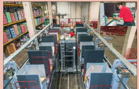
KNAPP’s Pick-It-Easy Move enables picking directly from pallets to roll containers.
