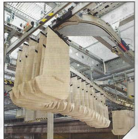
Using a 3-step matrix sortation process, the pockets are sequenced for the packing stations.
