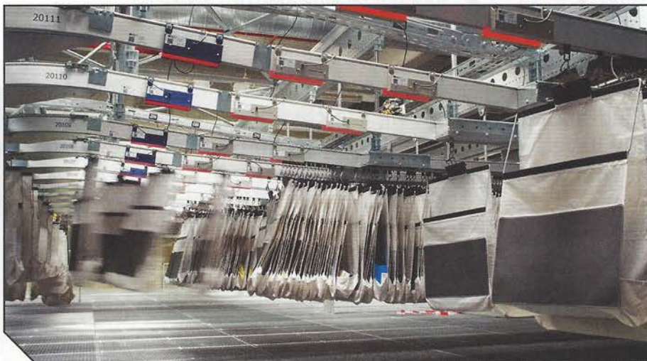
Each pocket is fitted with an RFID transponder so goods can be identified at any time.
