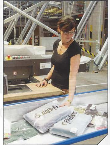
Warehouse operators push goods over a scanning area and into the pocket.
