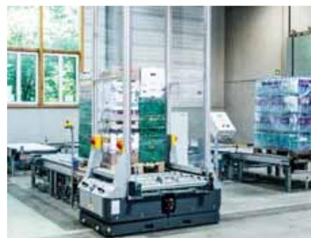
**S** PAR in Austria is operating a semi-automated solution from KNAPP that enables goods to be picked directly from pallets to roll containers.
