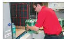
The workstation is designed so that goods can be pushed rather than lifted.
