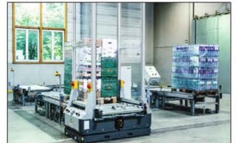
KNAPP's free-rooming Open Shuttles can transport pallets weighing up to 1300kg.
