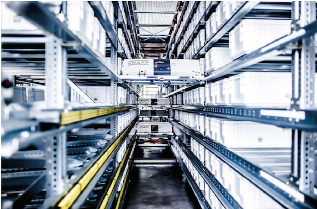
*With the OSR Shuttle™, every article in storage is ready for picking – ©KNAPP*
