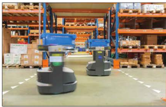
The Open Shuttle driverless vehicles use swarm intelligence.
