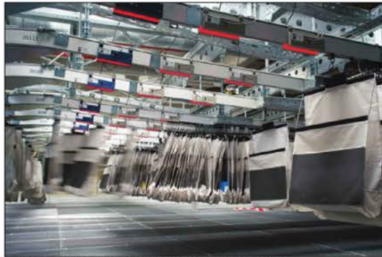
A three-step matrix sortation process is used to sequence the pockets.
