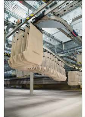
Each pocket has an RFID transponder so goods can be identified in the system at any time.
