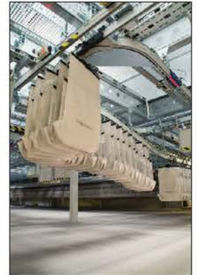
Each pocket has an RFID transponder so goods can be identified in the system at any time.
