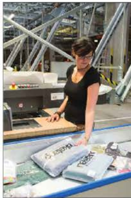
Warehouse staff push goods over a scanning area and into the pocket.
