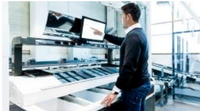
multichannel environments at which flat-packed goods can be placed into sorter pockets. Operators take articles – such as film-wrapped garments, shoes, books and DVDs – from the transport container and move them over an integrated scanner. When the item is scanned, the confirmation is displayed through a light signal in the adjacent chute, through which the goods
