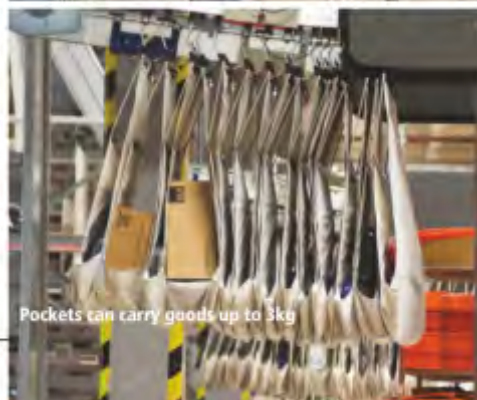
Each pocket has an RFID transponder
