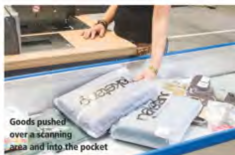
Three-step matrix sortation process sequences the pockets
