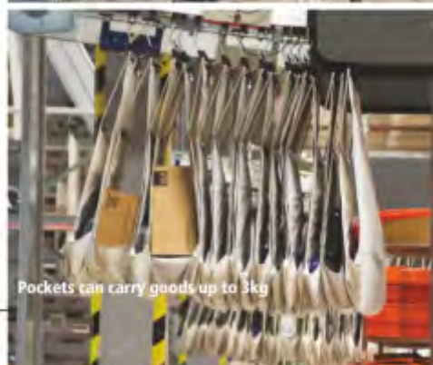
Each pocket has an RFID transponder
