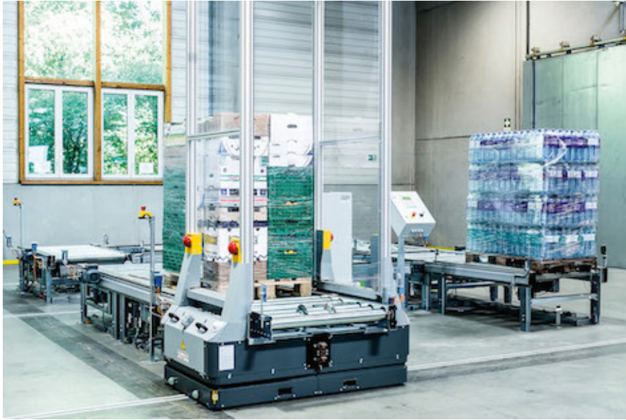
The driverless Open Shuttles for pallets transport loads weighing up to 1300 kg, navigating autonomously through the warehouse
