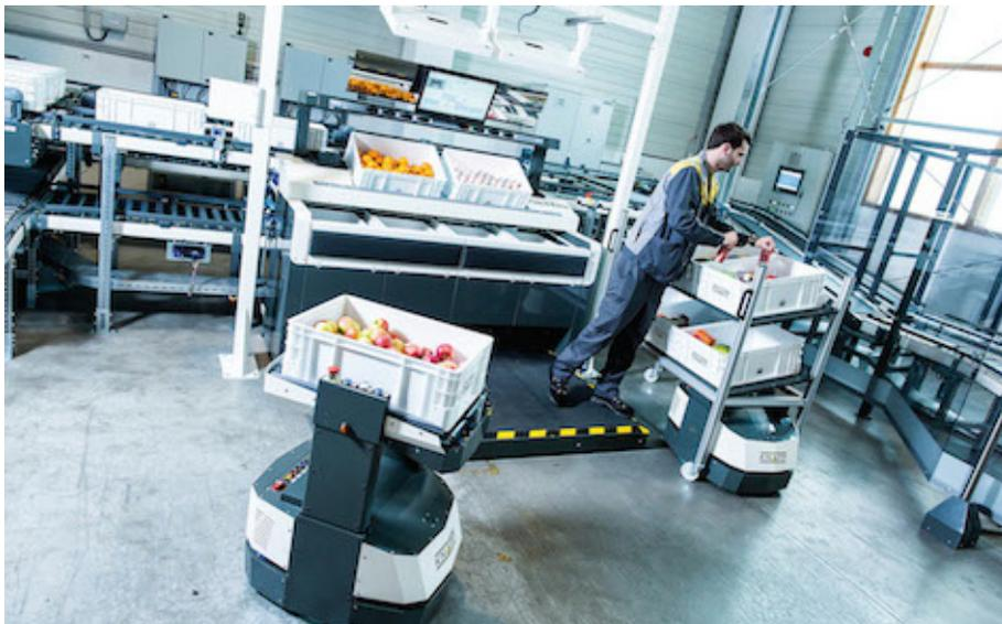
*Working on the principle of swarm intelligence, KNAPP's free-moving Open Shuttles can be used flexibly within the warehouse for transport tasks and to supply workstations*
